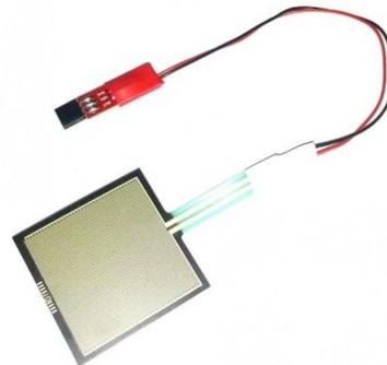
Fig. 6. Pressure Sensor [5]
