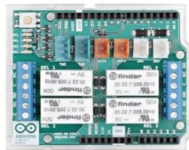
Fig.7. 4 Module Relay [6]
