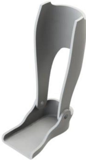
Fig. 3. The CAD model of the active orthoses realized in Solidworks 2016
